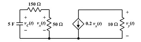
Given  $v_c(0) = 100$  V: (a) Determine  $v_y(t)$  for  $t \ge 0$ .
